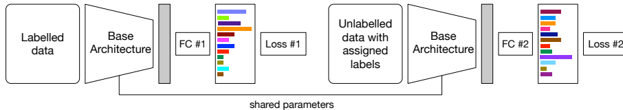
Fig. 3: Model updating in multi-task fashion. The weights of two CNNs are shared. “FC” denotes fully-connected classifier. In our experiments we use weighted Cross-Entropy loss as the objective.
